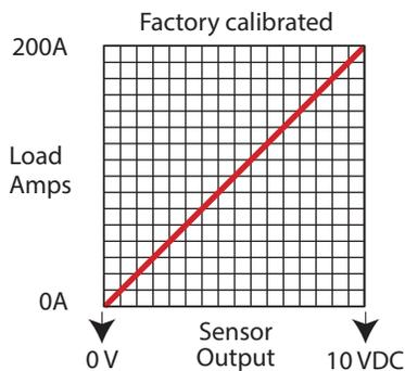
The C-2344-200 provides a 0-10vdc output signal proportional to monitored current to 200A full-scale.
